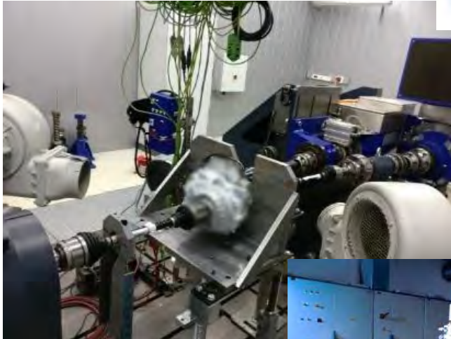
eDrive drivetrain testing with 250kW emulator
