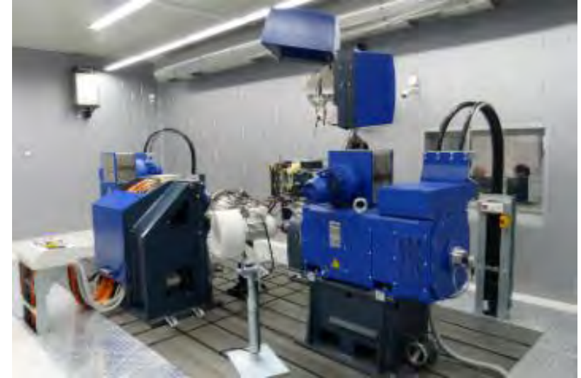
eDrive gearbox testing
