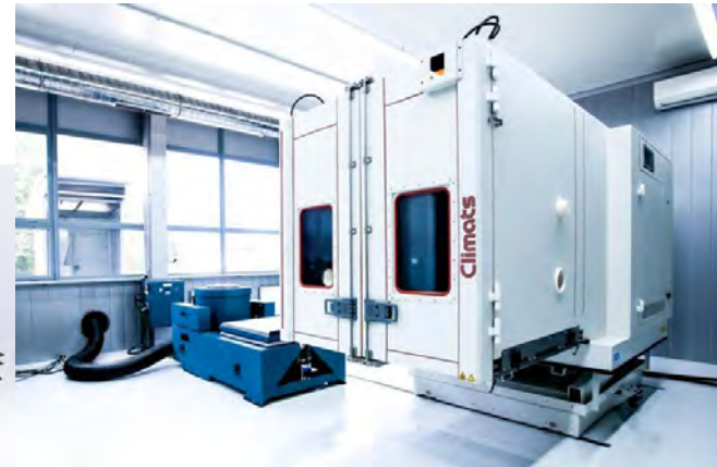
vibration stands with climatic chambers
