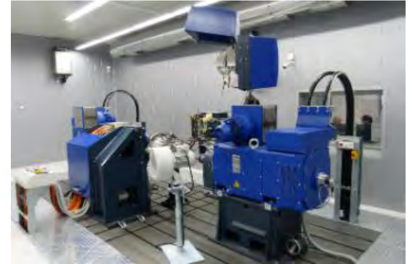
eDrive gearbox testing
