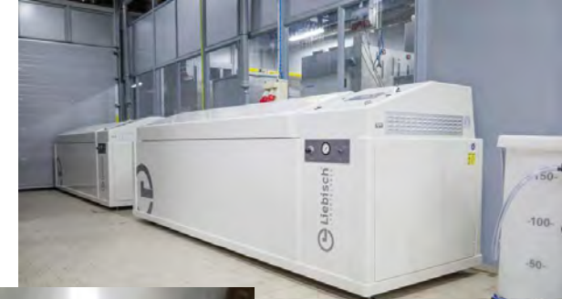
Large-dimension climatic chamber 3x7x9 m
