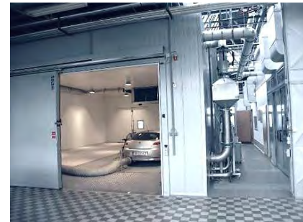
Climatic chamber (-35°C to +60°C) 14,3×10,1×4,3 m
