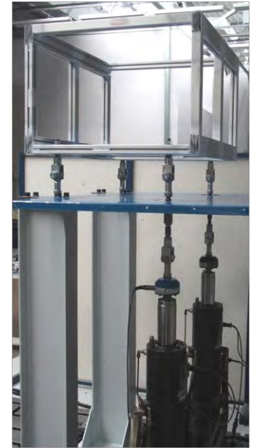
Durability test – multiaxial load
