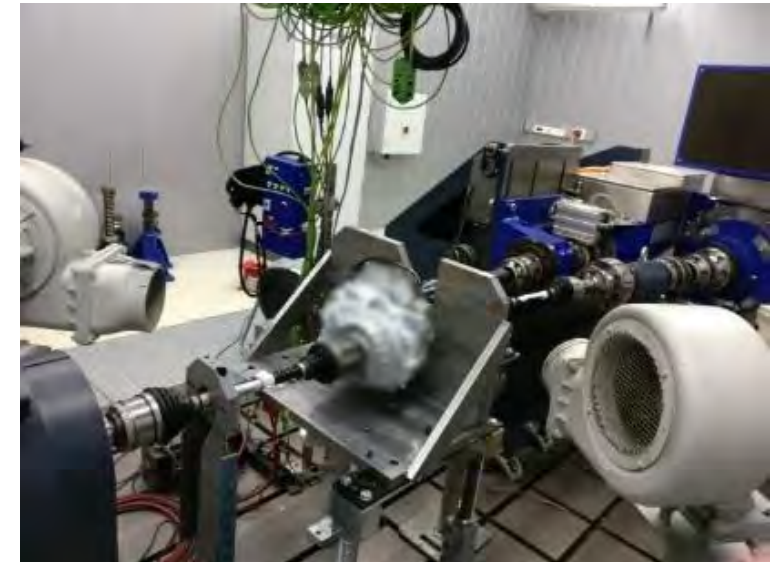
eDrive gearbox testing
