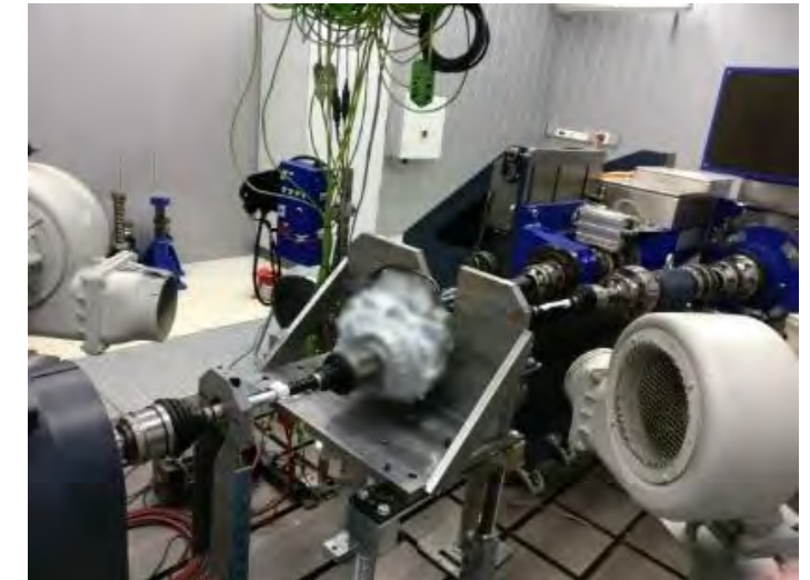
eDrive gearbox testing
