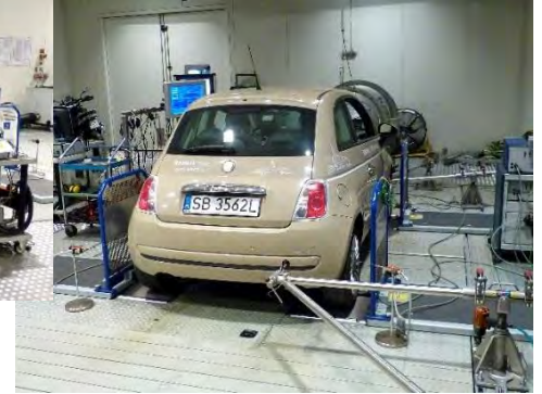
Large dimension climatic chamber Temp.: -45°C - + 75°C
