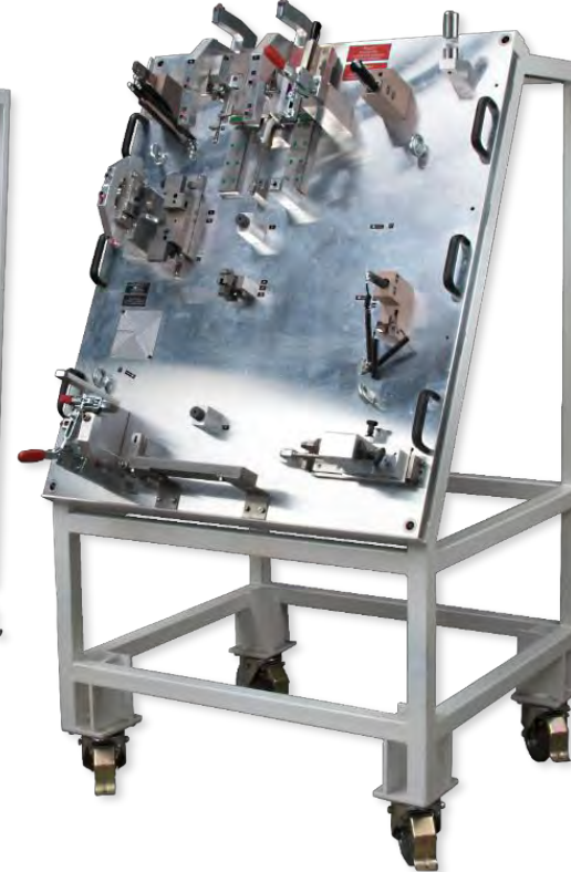
Checking fixtures for automotive seats
