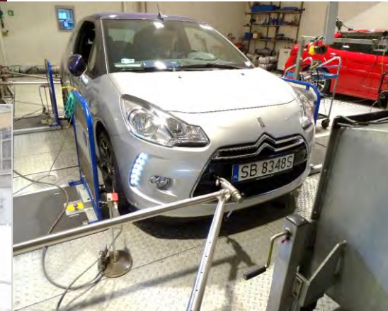
Vehicles tests in Temperature chamber
