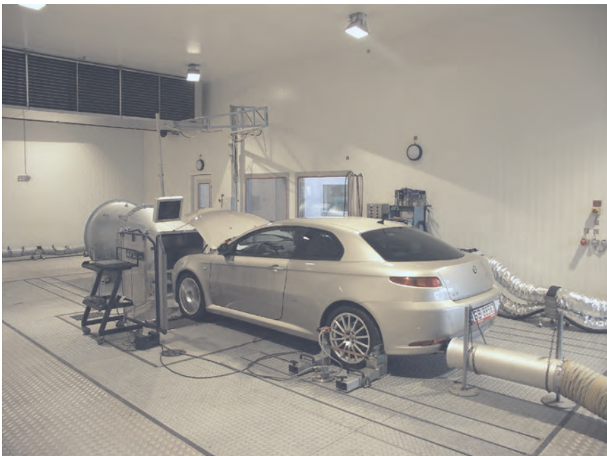
Fig. 5. Internal view of BOSMAL's new Euro 5/6 emissions testing laboratory, within a 620\text{ m}^3 climatic chamber
